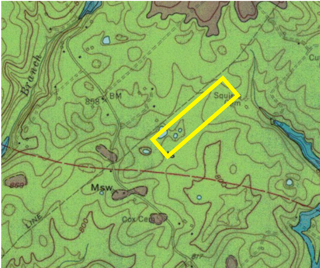
Image of the USGS Cane Valley Geologic Quadrangle showing the mapped sinkholes at and near the site (site is shown in the yellow rectangle).
